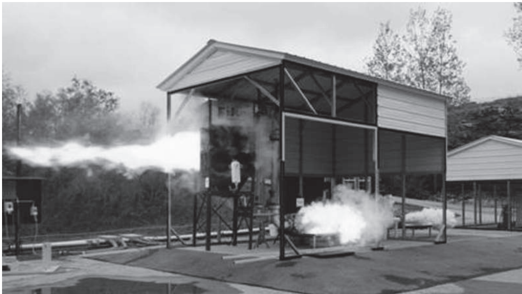
Figure 11.23. Dust collector explosion venting (Fike)
