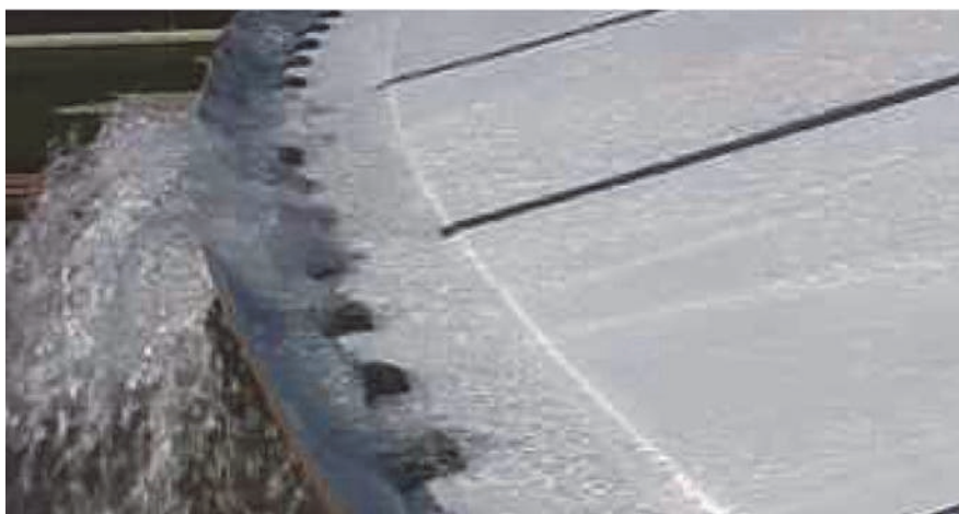
Figure 11.4. Breakup of liquid into drops spilling from tank top (Buncefield 2008)
