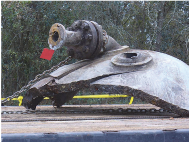
Figure 5.1. Portion of 7.6 cm (3 in)-thick reactor (CSB 2009)
