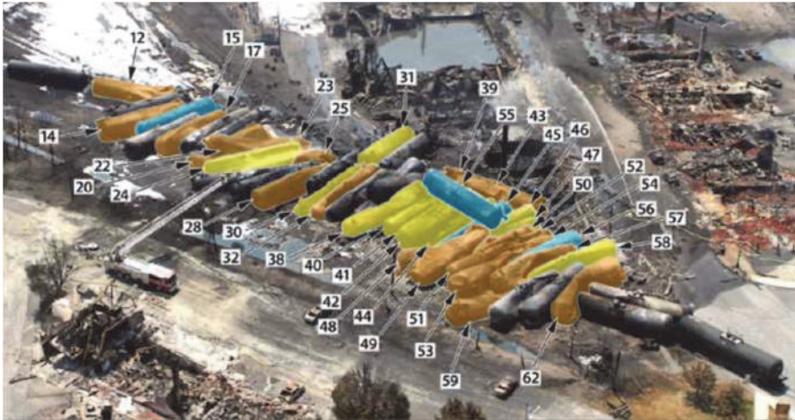
Figure 3.1. Lac-Mégantic tank cars with breaches to their shells (TSB 2013)
